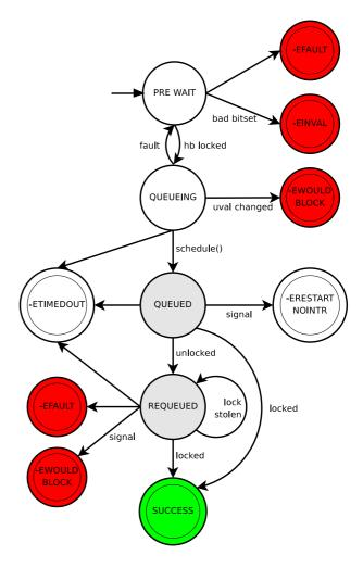
**FIGURE 6:** State transition diagram for futex\_wait\_requeue\_pi().
