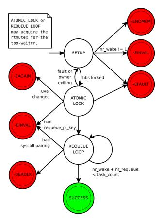
**FIGURE 7:** State transition diagram for futex\_requeue().
