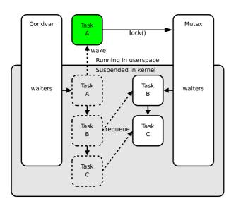
**FIGURE 2:** Thread state after pthread\_cond\_broadcast() (non PI case).
